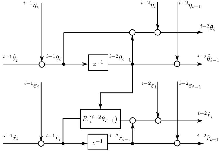
Figure 4: Block diagram of the considered state space model
