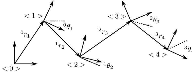
Figure 1: Sequence of positions-orientations attained by the vehicle
