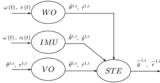
Figure 9: Improving the State Estimator
