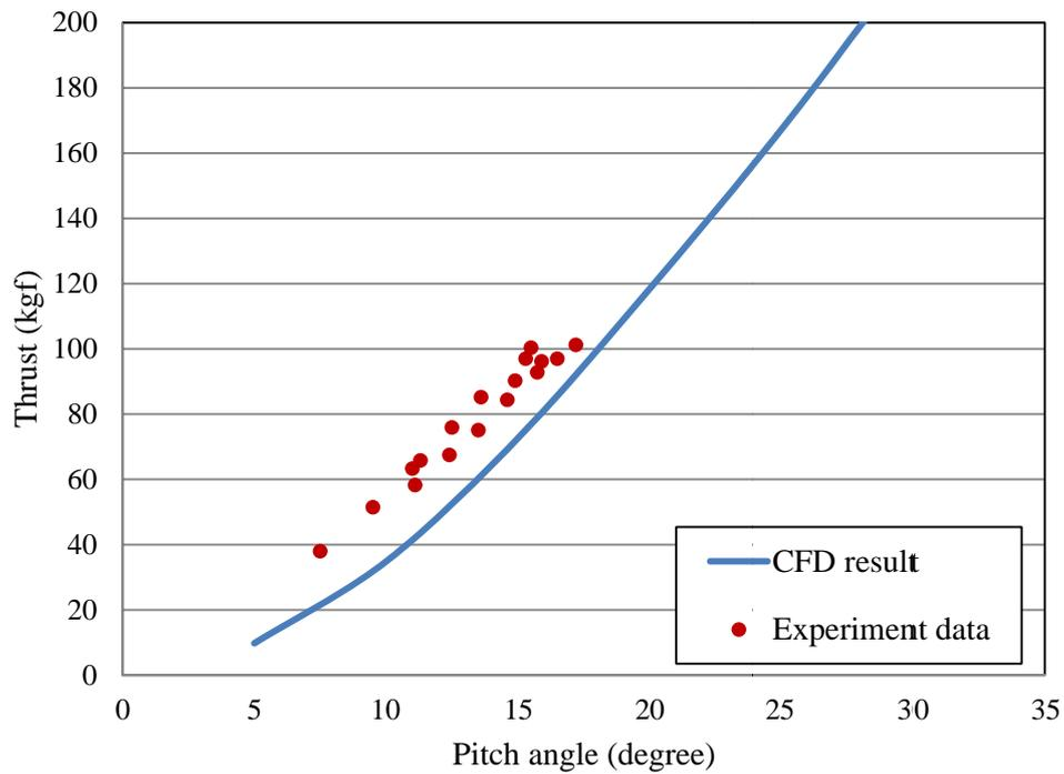
Figure 11: Experiment data vs. CFD result (main rotor only)
