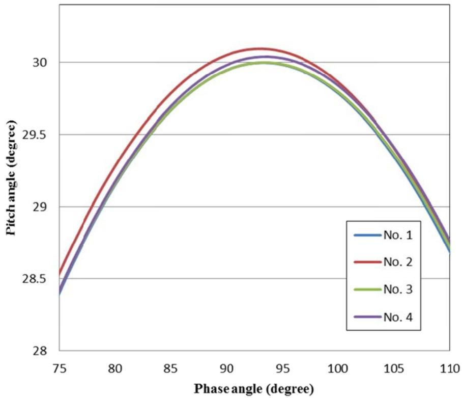
Figure 7: Pitch angle path of cycloidal blade system
