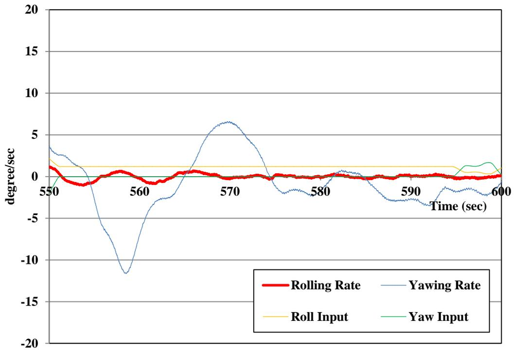
Figure 14: Graph of the rolling and yawing motion (stable)
