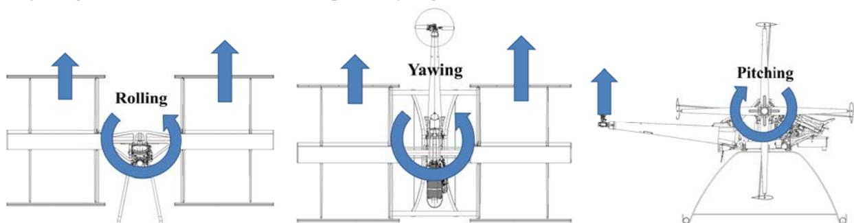
Figure 5: Scheme of attitude control of two-rotored cyclocopter
