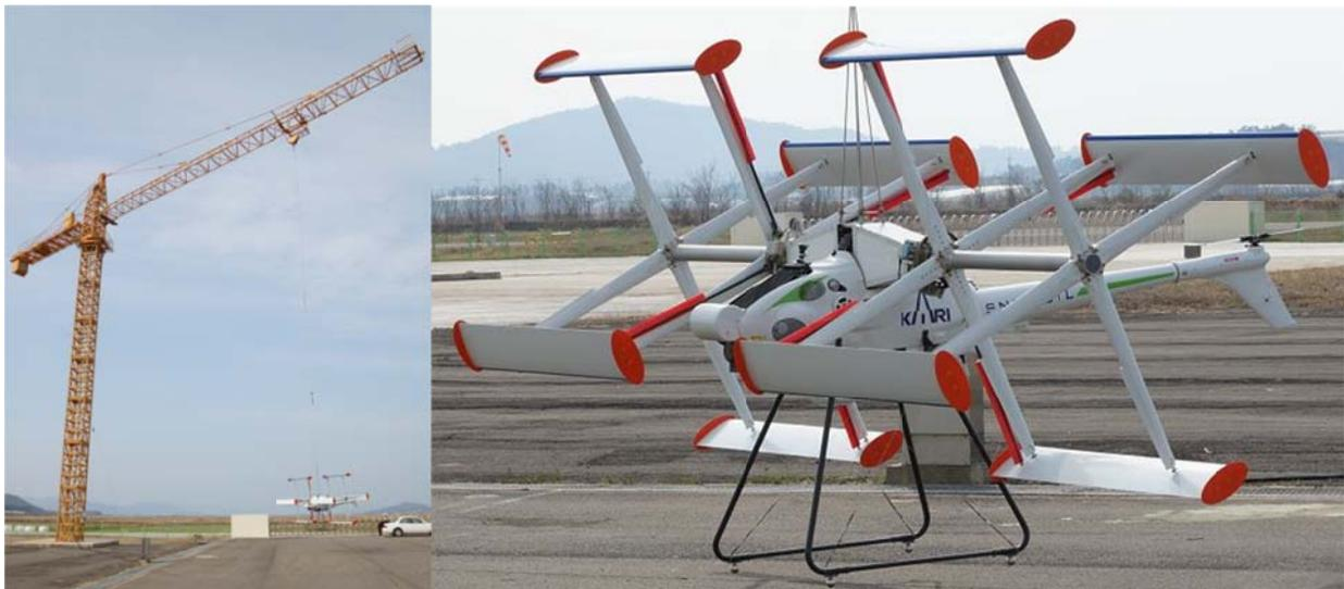
Figure 12: Tethering flight test
