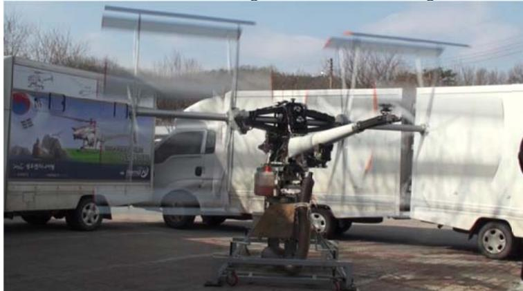
Figure 10: Ground test of the cyclocopter
