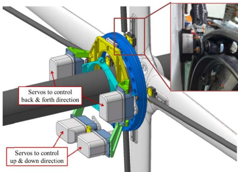
Figure 9: Control mechanism of new designed UAV cyclocopter
