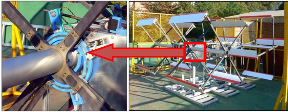
Figure 8: Control mechanism of previous UAV cyclocopter
