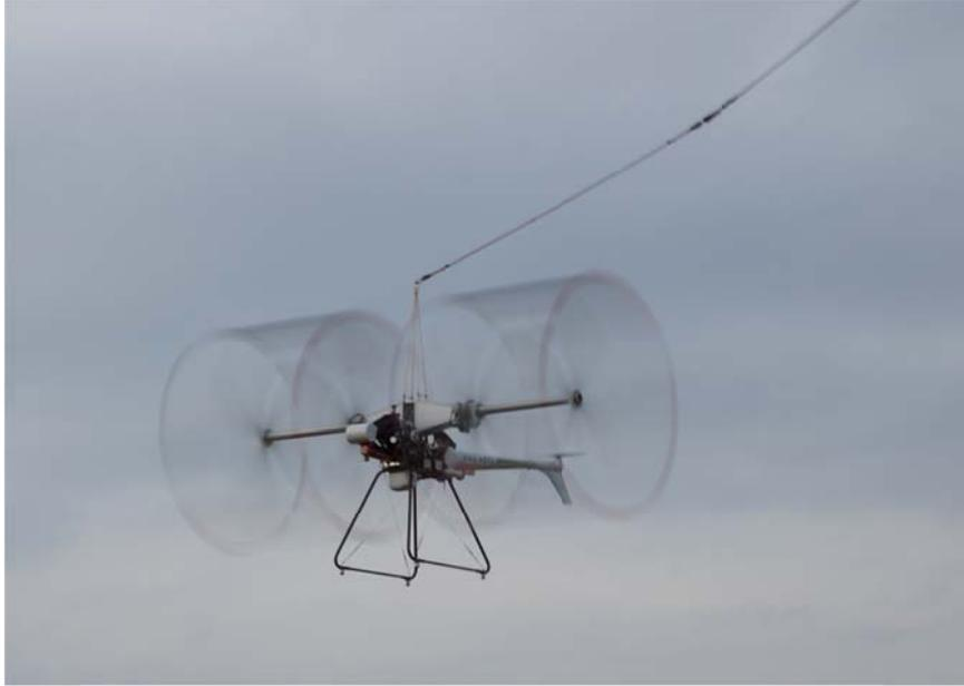
Figure 15: Stable hover flight of cyclocopter
