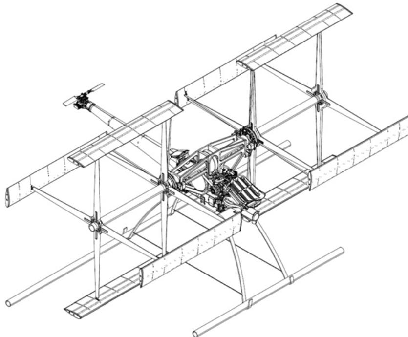
Figure 3: Designed cyclocopter
