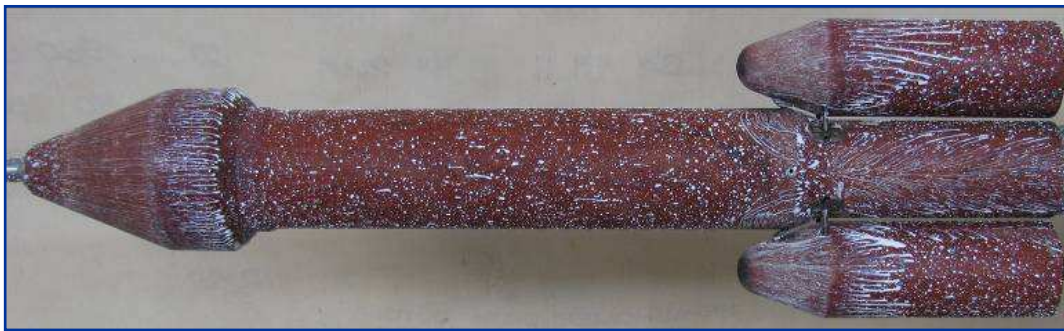
c) model MLV-R at \alpha=0 , M_\infty=7.5 , Re_{\infty,L}=6 \times 10^6 .
