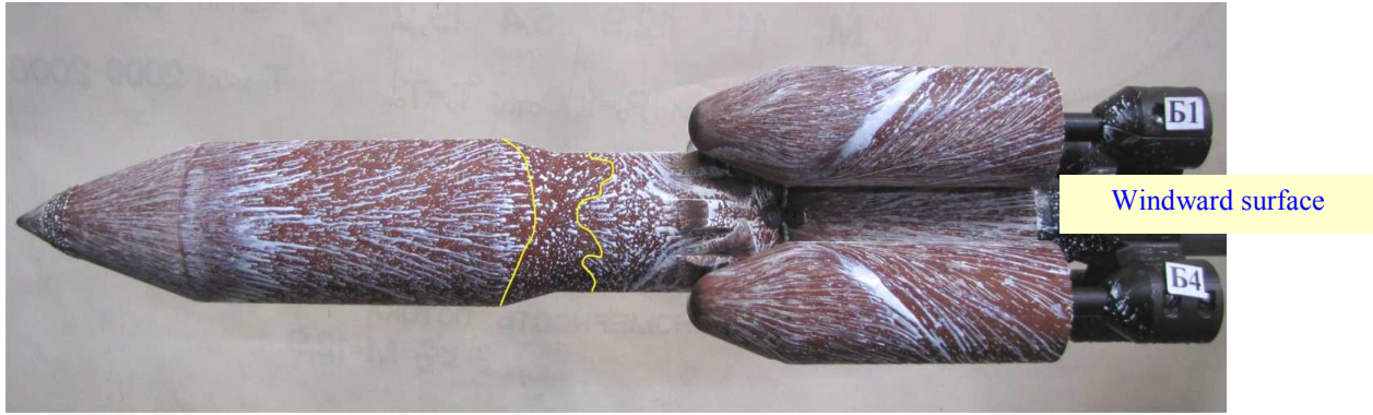
a) model MLV-A5 at \alpha=10 , M_\infty=7.5 , Re_{\infty,L}=5.5 \times 10^6 .
