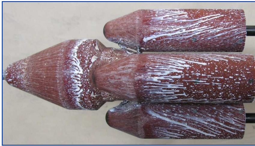
b) model MLV-A5P at \alpha=0 , M_\infty=7.5 , Re_{\infty,L}=5 \times 10^6 .
