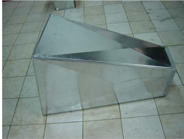
Figure 4: Contraction cone or nozzle of the constructed wind tunnel (longitudinal view).
