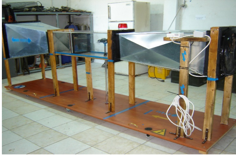
Figure 9: Fully fabricated subsonic, open circuit wind tunnel.
