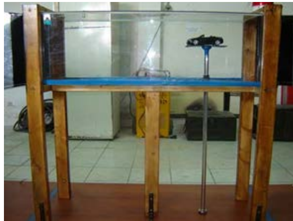
Figure 6: Test section of the constructed wind tunnel (longitudinal view).
