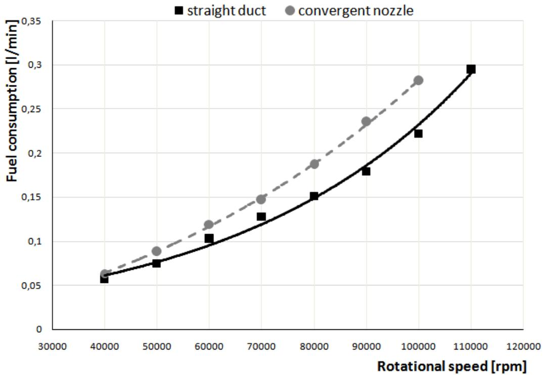
Figure 9: Fuel consumption as a function of engine speed
