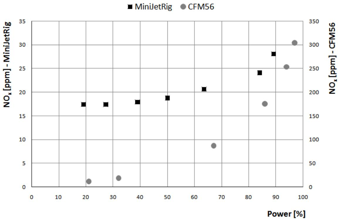
Figure 16: NO<sub>x</sub> emission for MiniJETRig and CFM56 [8]
