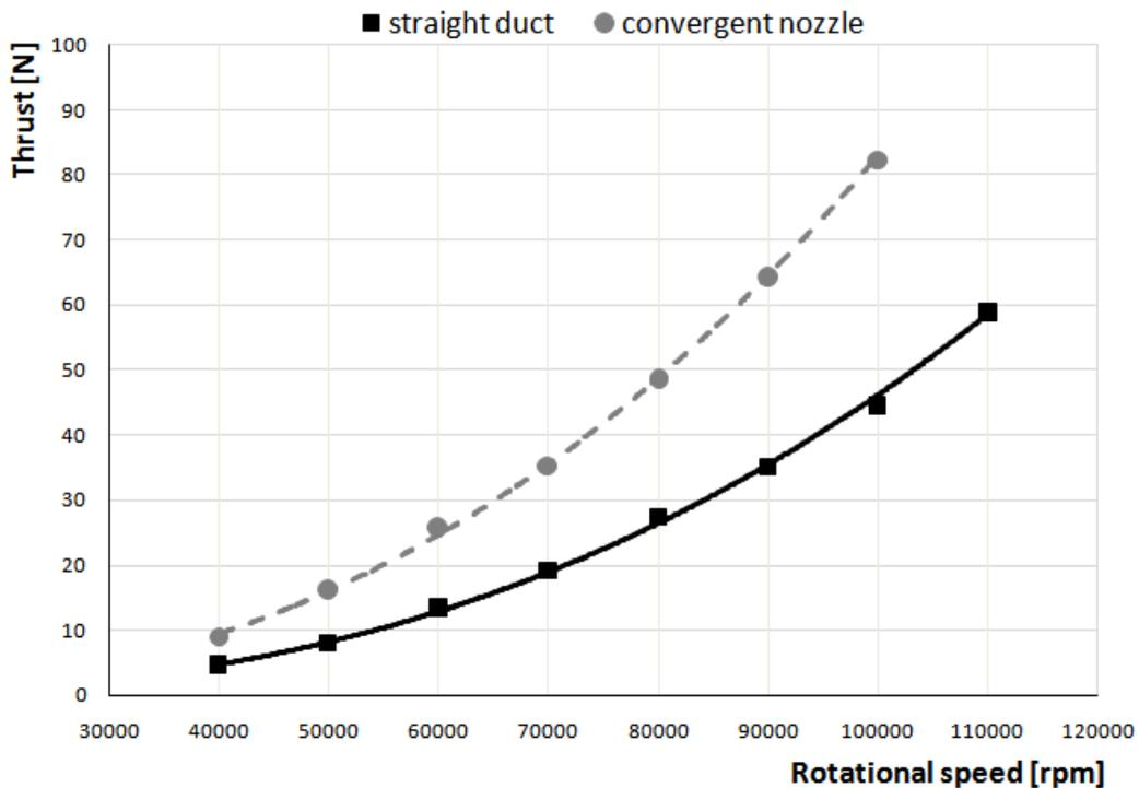
Figure 8: Thrust as a function of engine speed
