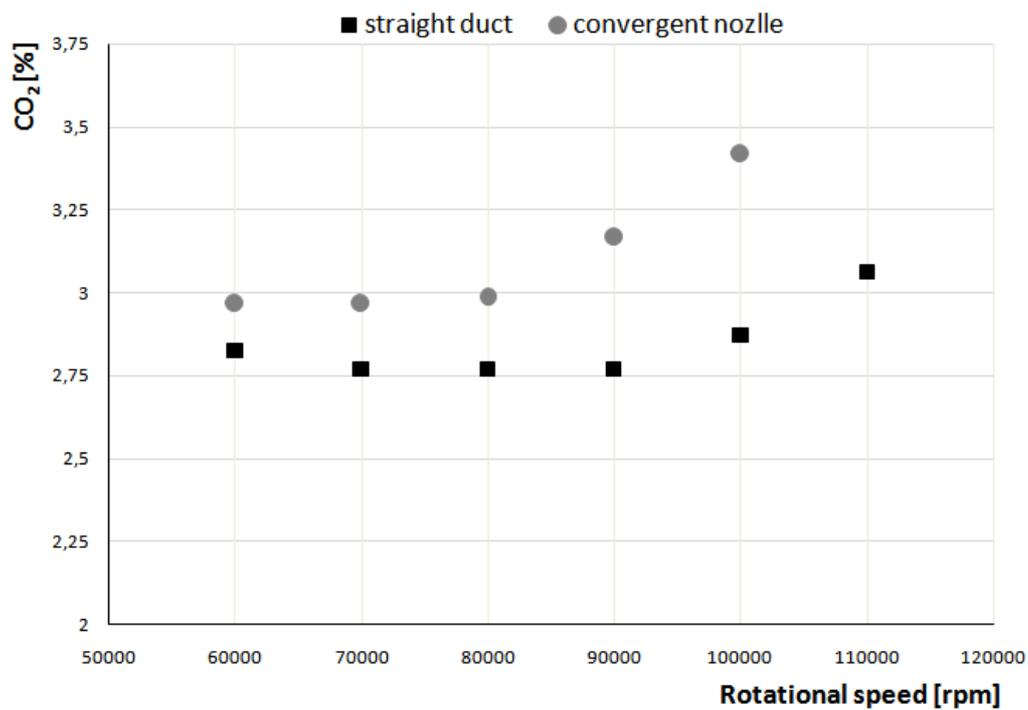
Figure 12: CO<sub>2</sub> emission as a function of engine speed
