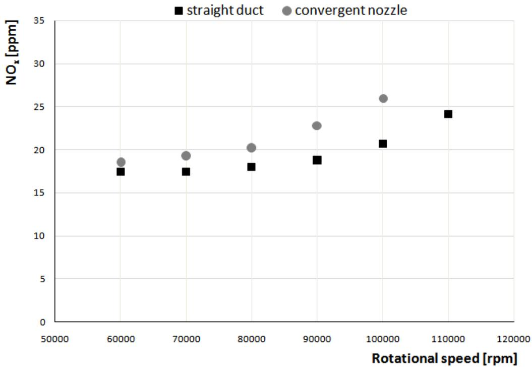
Figure 13: NO<sub>x</sub> emission as a function of engine speed
