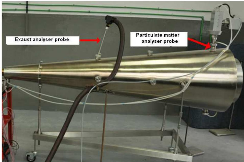
Figure 5: Measuring collector
