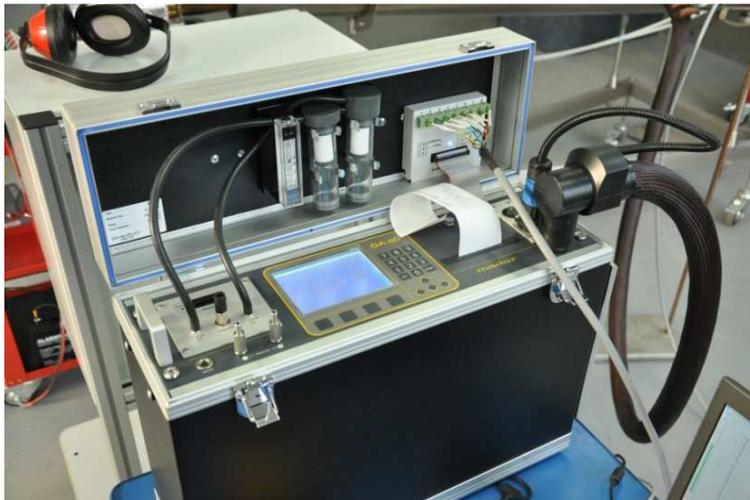
Figure 3: The exhaust analyser
