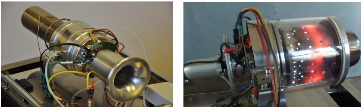
Figure 2: The miniature jet engine in two versions: metal and glass housing
