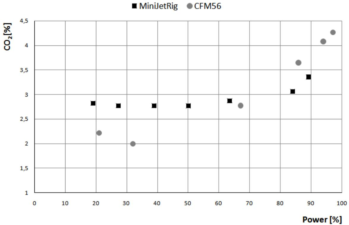
Figure 15: CO<sub>2</sub> emission for MiniJETRig and CFM56 [8]
