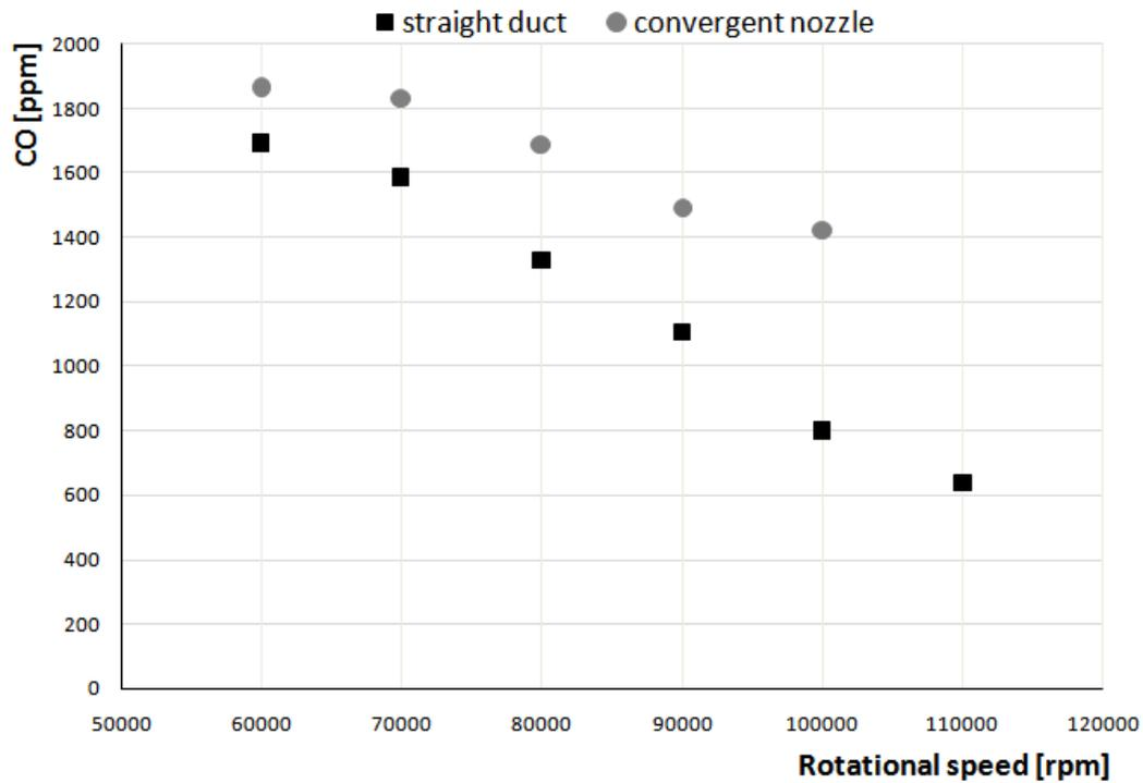
Figure 11: CO emission as a function of engine speed
