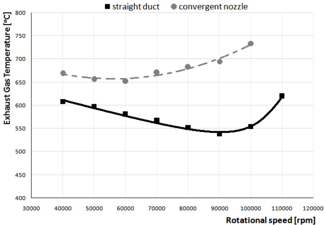
Figure 10: Exhaust Gas Temperature as a function of engine speed
