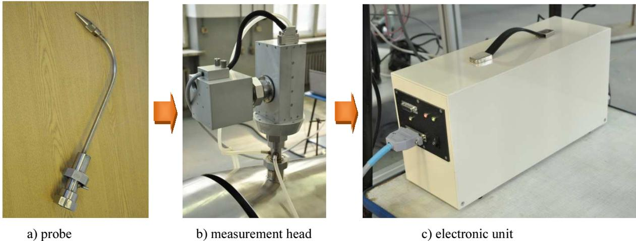
Figure 4: The analyser of particulate matter
