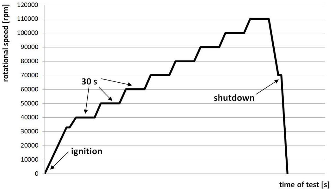
Figure 7: Profile of the engine test
