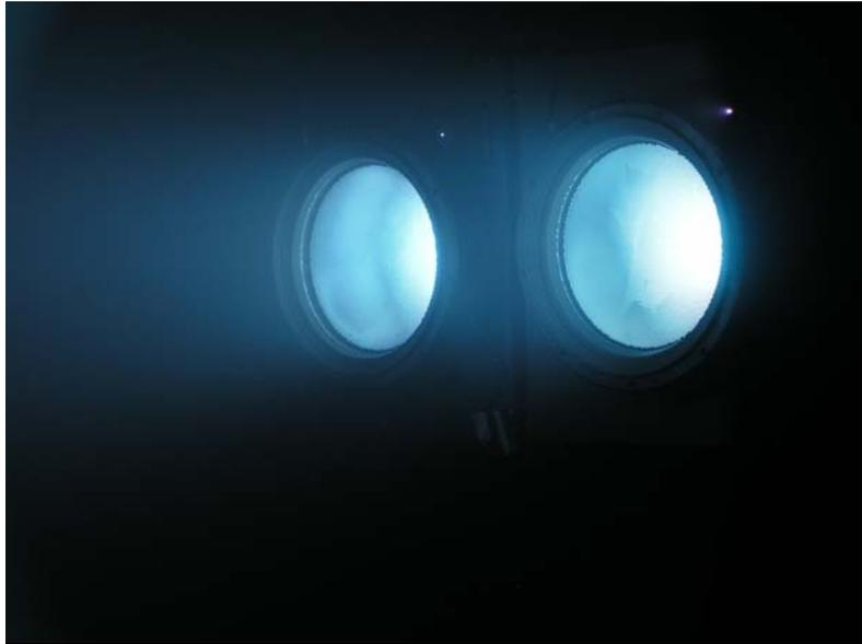
**Figure 10 RIT-22 during simultaneous operation of two thrusters**
