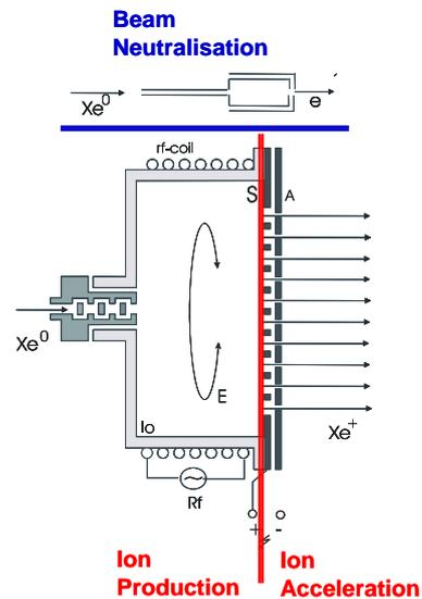
**Figure 1 RIT Operation Principle**
