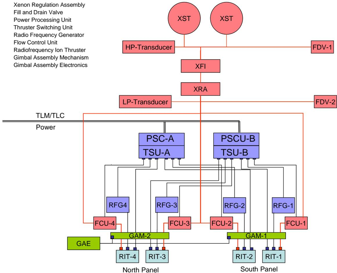
**Figure 12 RIT based propulsion system for station keeping**
