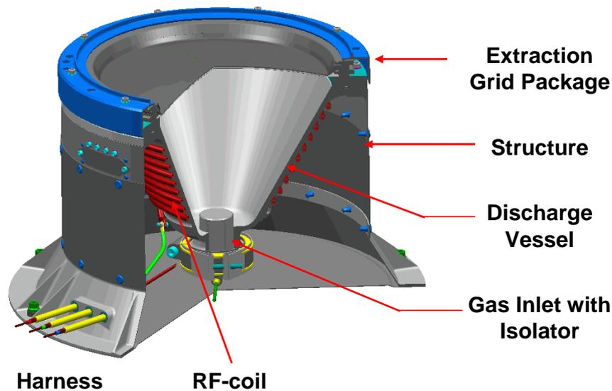
**Figure 2 RIT-22 explanation of components by means of 3D model)**
