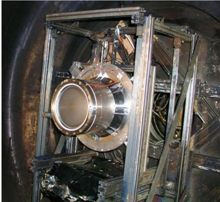
**Figure 11 RIT-22 EM installed in thrust measurement device**
