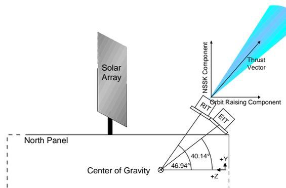
Figure 7: Ion Thruster Orientation ARTEMIS
