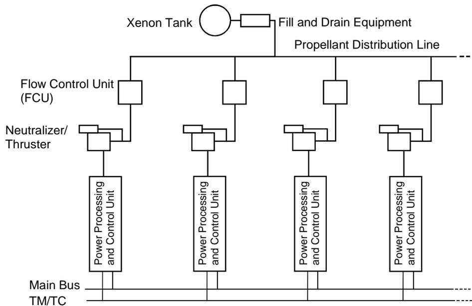
**Figure 13 ISS Orbit raising System Block Diagram**
