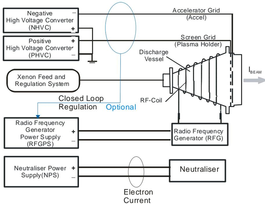
**Figure 3 RITA System Block Diagram**
